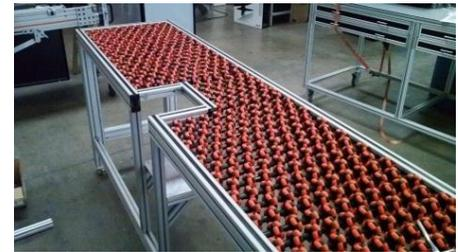
The new workstation met all expectations for increased productivity and improved ergonomics. The need to lean, twist and pull has been completely eliminated. The heavy Silflex™ radiation shielding blankets are now maneuvered and positioned easily with one hand in all directions.
